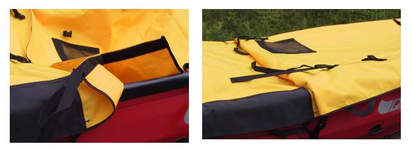
**e.** Lace the center section. Keep in mind that the stern paddler may need to access gear while under way. It should be possible to open the cover between sections by undoing the straps (two on top and two securing the edges to the cord that is attached to the hull), but without undoing any lacing.
