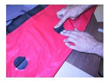
Move back to the first patch you installed, flip the template over and start working towards the other end of the canoe.
